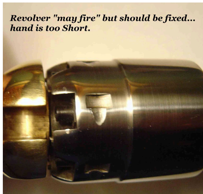
Picture 3: Shows the timing way off also when the cylinder looks like this at full cock it is telling you the hand is too short.
